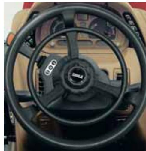
▲ **Industry-leading maneuverability with the Turn Assist option.** Normally, turning the front wheels from one side to the other requires four turns. With Turn Assist, simply push the inside ring, and full left or right turns can be made by turning the steering wheel just 10 degrees left or right, reducing operator effort and increasing productivity.
