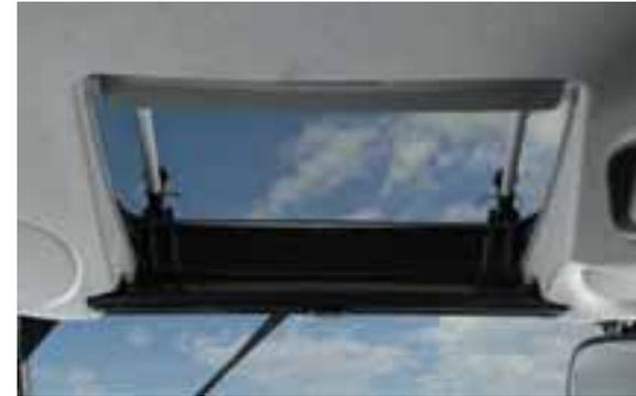
▲ **High-visibility roof window** offers exceptional view of the loader at work in the raised position.
