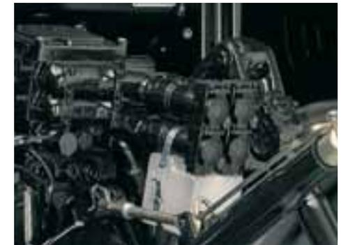
▲ **Two dedicated pumps** – one with 40 lpm for steering and lubrication, and one with up to 113 l/min with CCLS pump for hitch and remote valves - provide reliable productivity and a maximum of 153 l/min total tractor flow.
